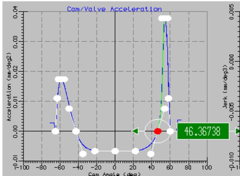
The highly asymmetric nature of this profile would not be typical but is intended to illustrate the process of matching highly unequal profile halves. As with all cam profile designs, irrespective of their maths origins, the profile should be checked for overall acceptable results. This particular example would almost certainly not be due to its high acceleration and jerk values.
