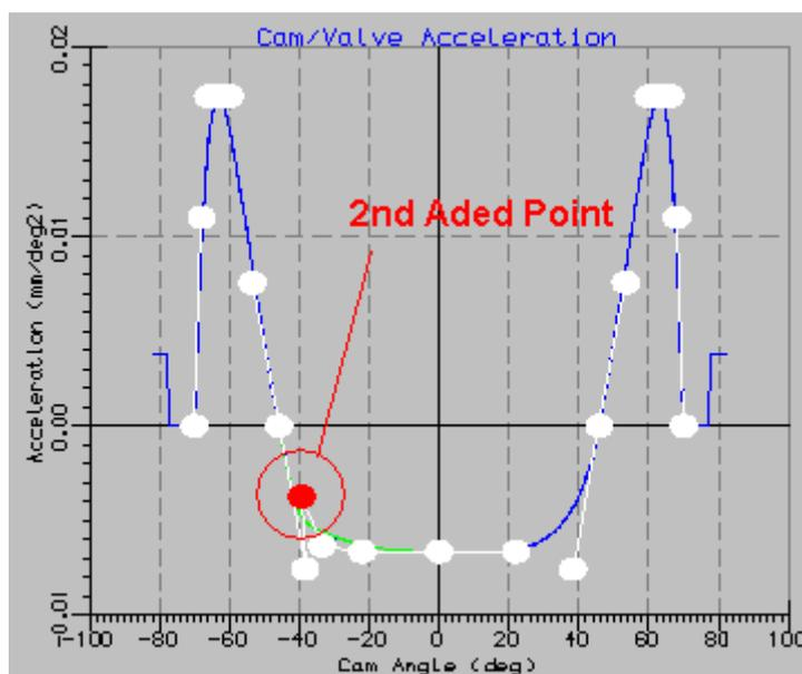
With these additional control points experiment with dragging them to assess the impact on overall control of acceleration shape. Note that initially the extra points are not mirrored across to the closing side. Once you modify any point, they additional points will be added.
