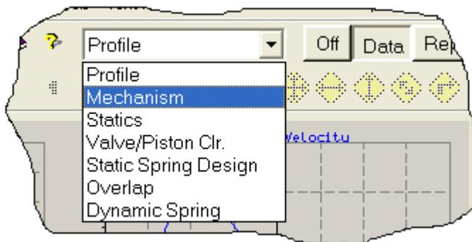
The model data is arranged under seven separate headings, **'Profile', 'Mechanism', 'Statics', 'Valve/Piston clr', 'Spring Design', 'Overlap' and 'Dynamic Spring'**. Go through each of these main options using the selection box located in the toolbar to review the data associated with each section.
