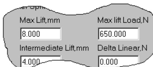
To produce a progressive rate spring, in the **Delta Linear** box enter **5.0**. Update the calculation. The rate results displayed for the fitted, interim and max lift conditions will now vary, increasing as the number of active coils reduces with lift.
