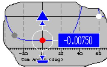
To change the value, select and hold down the **Ctrl** key, then press the **Up Arrow** or **Down Arrow** key to move the point. This 'joggles' the point in coarse steps. To change to joggle with the fine step size, select and hold down the **Shift** key, then as before press the **Up Arrow** or **Down Arrow** key to move the point. The cam profile calculations are updated with each joggle step.
