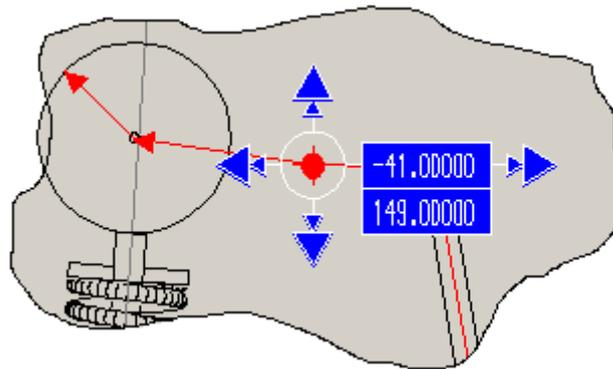
Try holding the **Ctrl** key down and use the **Up, Down, Left** and **Right** arrow keys to move the pivot points position.
