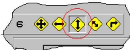
We can now run the auto-match, from the menus select **Solve / Bezier Options / Match Velocity at Max Lift**. This will perform a number of checks on point selection before starting the matching process. Our selected point will now be moved up and down in the y-direction automatically hunting for the position that gives us the zero-velocity value. The 'hunting' process continually refines the step size to home in on a solution within our specified tolerance.
