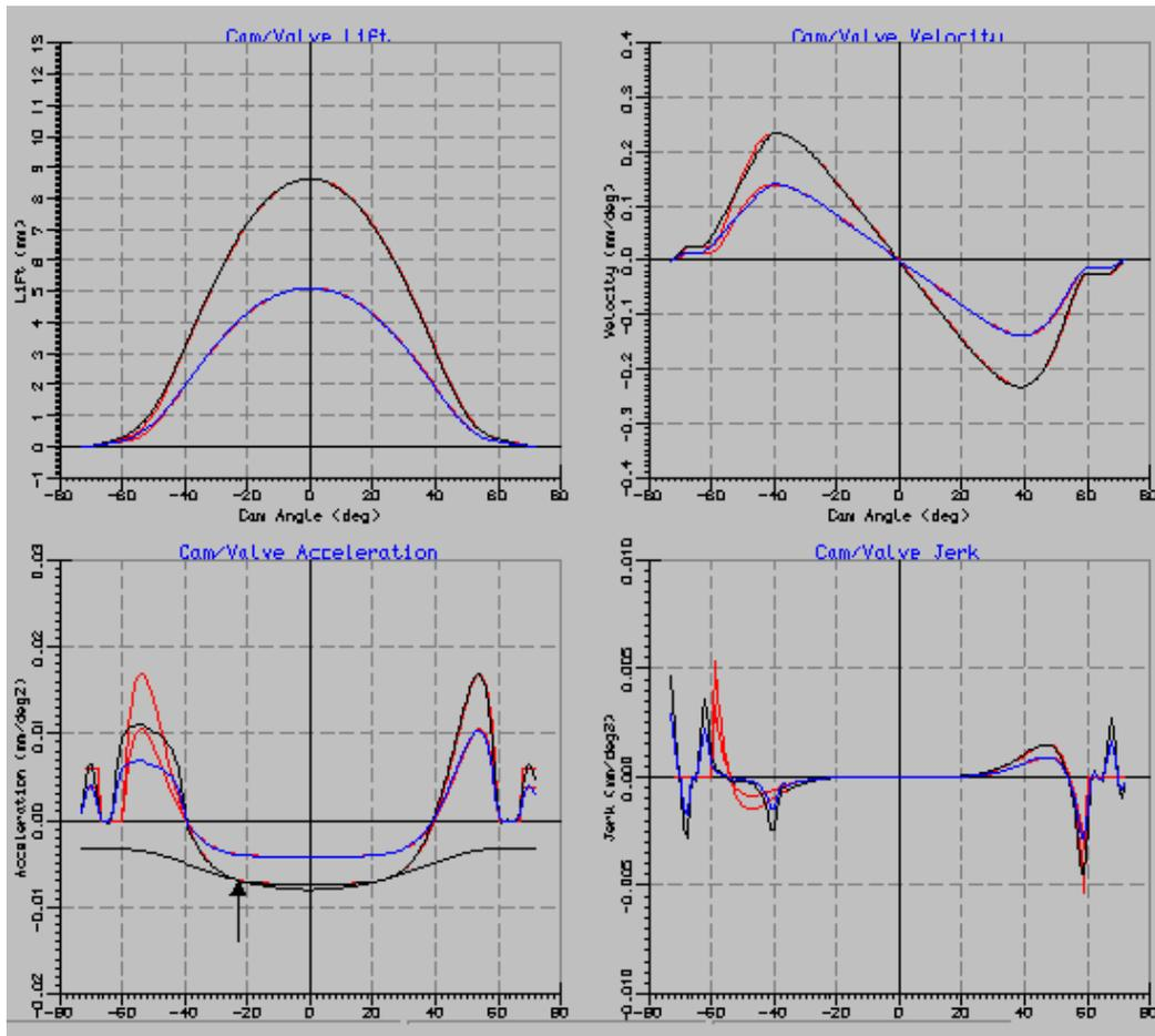
Comparison of Profile before (red) and after (blue/black) the concavity tool
