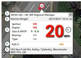
Number of Satellites & HDOP (Horizontal Dilution of Precision). A minimum of 3 satellites is required for a fix. HDOP is a measure of the geometric quality of the satellite configuration in the sky. HDOP is a factor in determining the relative accuracy of a horizontal position. The smaller the DOP number, the better the geometry. We would expect a HDOP value to always be less than 2.0 for a good 3D fix
